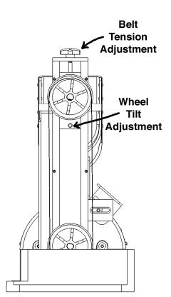
Remove the old belt, if one is installed, by sliding it off the upper and lower wheels.
